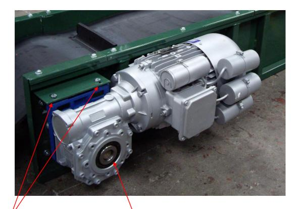
Bolt gearbox onto mounting bracket
