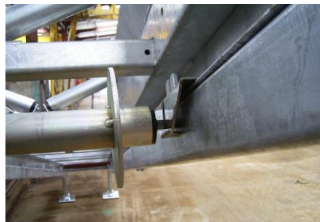
Disc Return Rollers fitted with stringers
