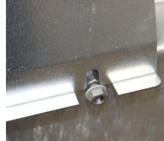
Cover slotted onto bolts
