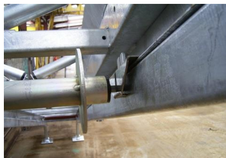
Disc Return Rollers fitted with stringers
