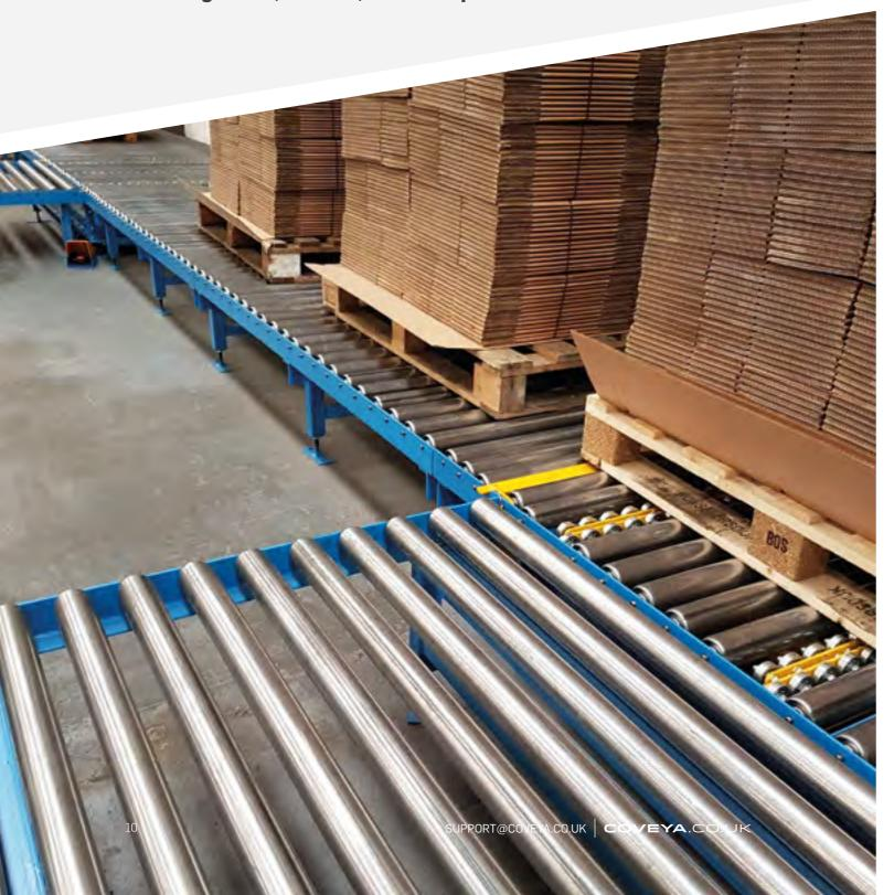
Products can be accumulated on a lineshaft conveyors, in other words held in a queue, without stopping the upstream movement of other products on the conveyor. This is possible because the drive mechanism design only generates low levels of line pressure. When products are stopped on the conveyor by a mechanical stop the rollers stop rotating and the corresponding O-rings to slip on their spools, without affecting any other rollers elsewhere on the conveyor.
